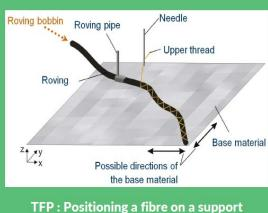
TFP : Positioning a fibre on a support material by stitching in any orientation
